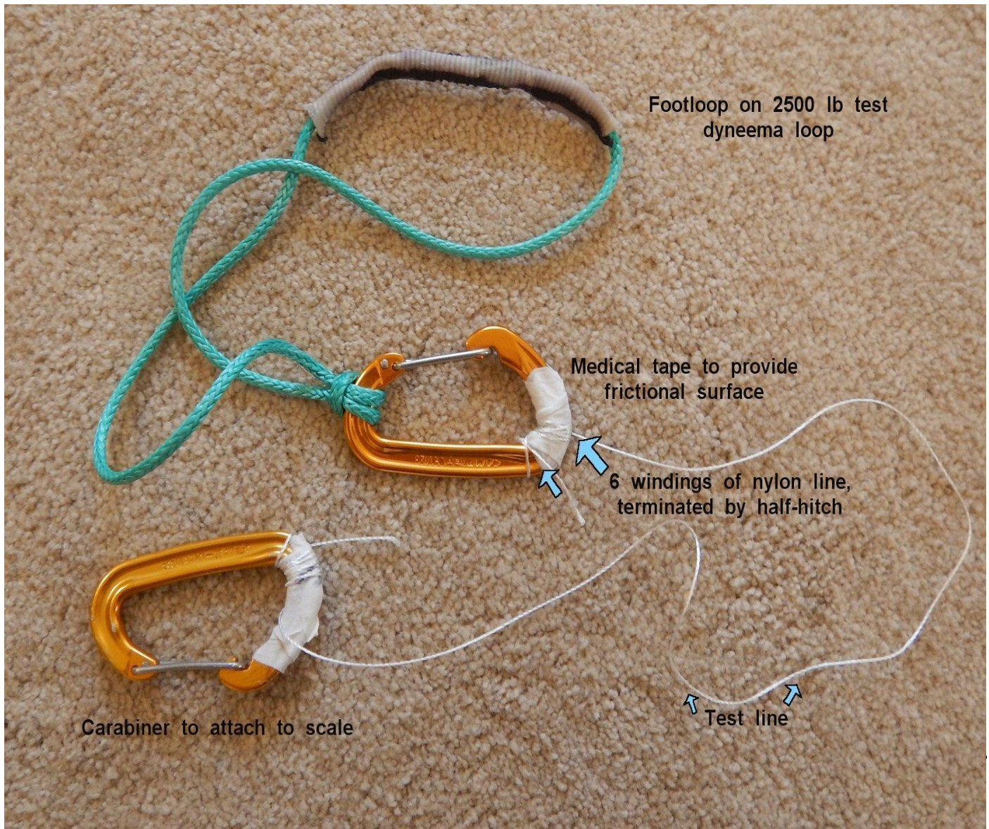
Figure 3. "Capstan" clamps using carabiners
