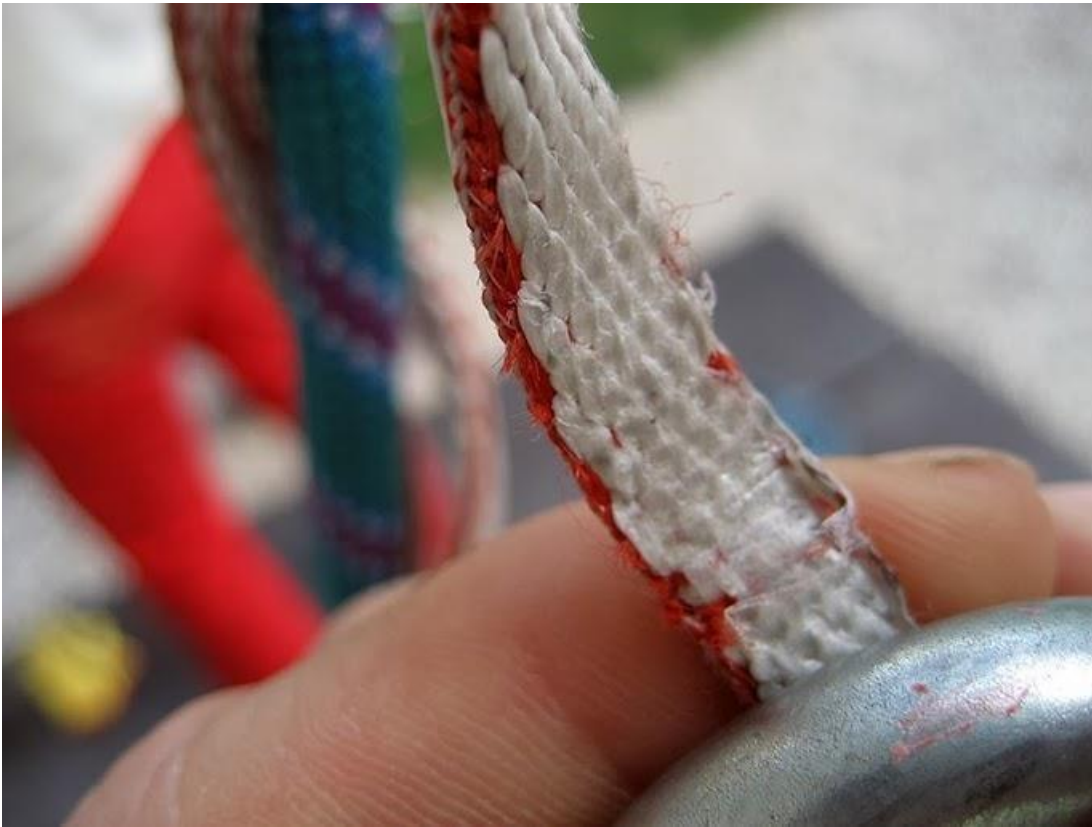
Figure 2. Rope desheathed by UIAA drop test.
