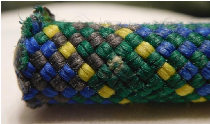
Figure 9. Nature of sheath on dynamic 10mm rope.
