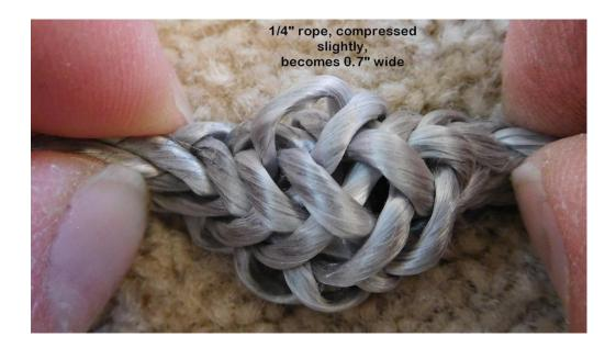
Dyneema Corporation has produced many types of the fiber, with different characteristics; some have been obsoleted. The more recent tend to be SK75, SK78, and SK99. Amsteel Blue is made from SK78; Marlow Ropes makes a similar cord from SK99. Both SK75 and SK78 have the same approximate breaking strength, but the more expensive SK78 has lower "creep." SK99 is relatively new, and is 15-20% stronger than SK78, and currently much more expensive.
