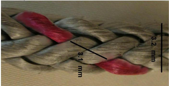
One strand has been marked pink; it starts on the outside of the rope, dives under two other strands where it is effectively in the "center," then remerges after on the surface just ~3mm later.
